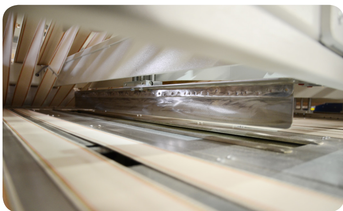
Reliable cross folding: Unifold has knife folding for all crossfolds.
